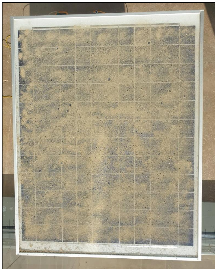
Figure 3.17 PV module with 30 g of dust accumulated on the front surface
